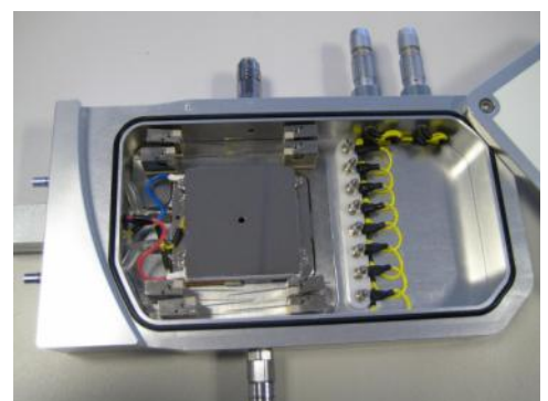
The LTS120E-PL8 Peltier heated/cooled probe stage with temperature range of -40^{\circ}\text{C} to +120^{\circ}\text{C} , fitted with spring post connectors and LEMO feed-through.
