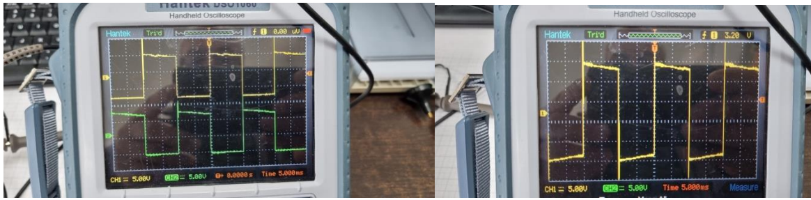
Figure 29. From left to right and from top to bottom: inverter diagram; experimental assembly; transistor drain signal and inverter output signal, respectively.
